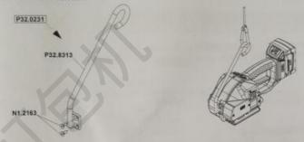
With the swivel mounted suspension bracket the package can be strapped in various working positions. The complete suspension bracket can be ordered under item number P32.0223.
